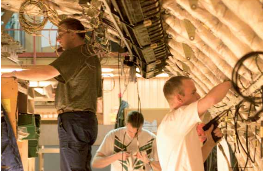
Complexity under control: Routing cables in the Airbus
